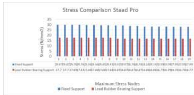
Figure 6: Stress Comparison Fixed vs Lead Rubber Bearing Support (Staad Pro)
